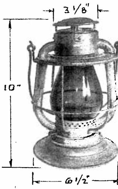
1904 TO MID-1905 THE 'THIRD VERSION' OF THE DIETZ VESTA RAILROAD LANTERN WAS INTRODUCED. IT WAS A TUBULAR DESIGN WITH RIDGED TWIST-OFF BELL BOTTOM. IT WAS MADE WITH A SOLID SMOKE DOME MOUNTED ON TABS CREATING WIDE SIDE OPENINGS.
